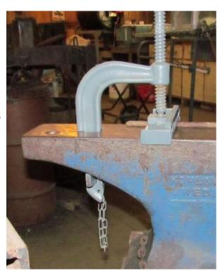
The image here shows the wedge that taps into place and locks the device in the anvil. The unit takes a couple of seconds to install and virtually the same time to use as the usual bent-rod-in-the-pritchel-hole tool but without the drama of sliding off the stock.
